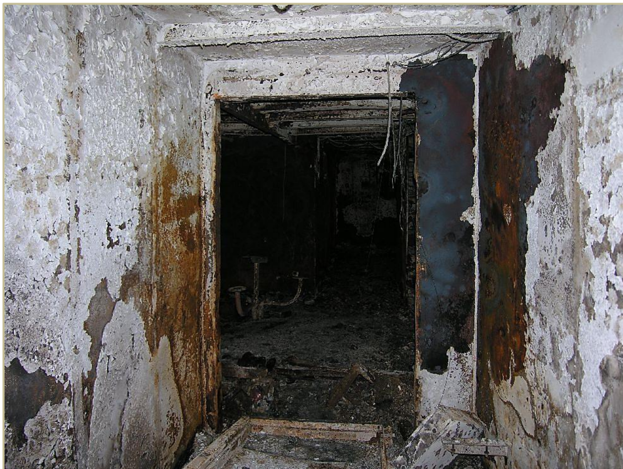
The steel door of the centerline passageway to the galley (main deck frame 25) is lying on the deck. The wooden door frame was consumed in the fire. Photo by TSB.
