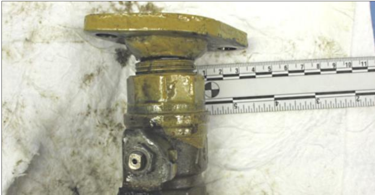
The assembly, as received. The crack was located along a thread valley and spanned across about 75 percent of the assembly's circumference.
